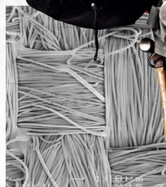
Photos above are Scanning Electron Microscope (SEM) >300X magnification showing front and side views of a typical 1000d air textured nylon CORDURA® Classic fabric.
